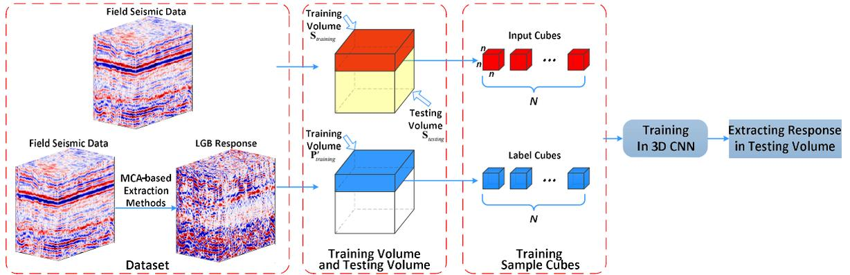
Figure 2: Proposed workflow based on 3D CNN for extracting LGB response. The training data are extracted as a subset from the field seismic data and the corresponding LGB response extracted by MCA-based method.
