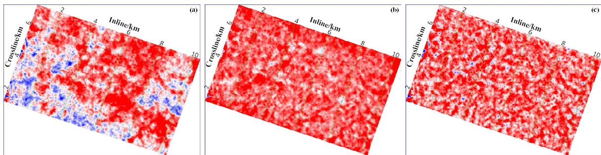
Figure 4: A time slice of the test result on raw seismic data from Eastern China. (a) Raw seismic data in deep layer in which weak-energy LGB waveform response is covered; (b) LGB seismic waveform response extracted by MCA-based method; (c) LGB seismic waveform response extracted by our method.
