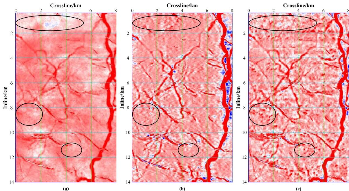
Figure 5: A time slice of the test result on another raw seismic data from Eastern China. (a) Raw seismic data; (b) LGB seismic waveform response extracted by MCA-based method; (c) LGB seismic waveform response extracted by our method.
