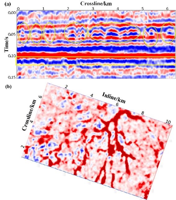
Figure 1: Raw seismic data. (a) Raw seismic section. The channel structures in shallow layer (indicated by yellow ellipses) are clear. However, the deep layer data are covered by the strong reflection layer, which makes it impossible to clearly depict the weak-energy LGB waveform response. (b) A time slice of 0.046s for training.
