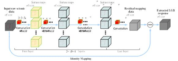
Figure 3: Architecture of the proposed 3D CNN for LGB features extraction.
